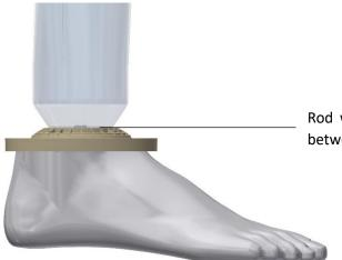
Rod welding (whole circumference) on the interface between the socket and the concave ankle washer.
