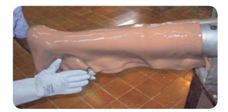
Tighten the polypropylene around the suction cone with a rope or something similar.
