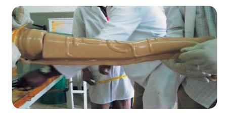
With scissors or a knife, cut off the excess polypropylene along the welding seam while it is still hot.
