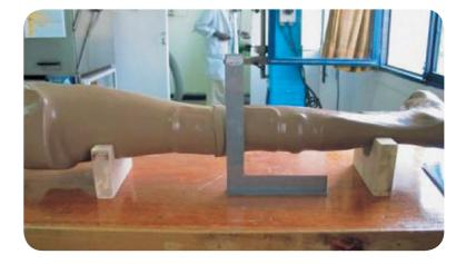
The position of the knee axis should be marked in relation to the vertical line indicating the location of the mechanical knee joint.
