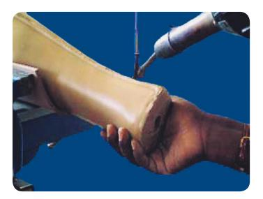
Weld the ankle to the shell. After welding, carefully flatten the ankle surface.
