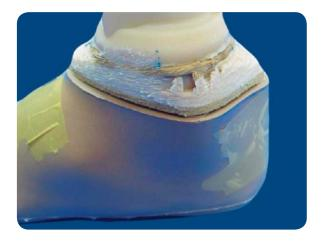
• Roughen the surface of the socket.
