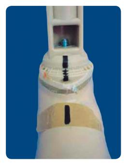
• Disassemble the foot and draw a line all around the plate 3 mm from the edge.
