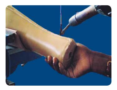
• Weld the ankle to the shell. After welding, carefully flatten the ankle surface.
