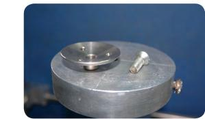
Install the heavy-duty nut in the centre of the jig
