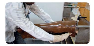
Add 10 mm of hot PP (square shapes of the same width as the mould)
