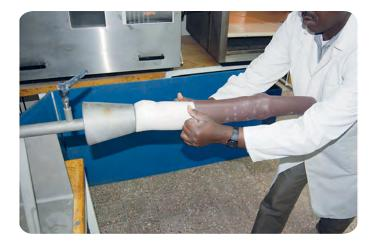
Cover the mould with a plastic bag and apply the vacuum
