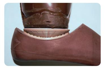
Use an oscillating saw to cut the medial window in the device
