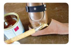
Fill the gap between the socket and the foot with EVA
