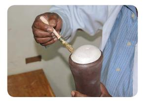
Heat the cap until malleable and apply it to the distal end of the positive mould; maintain constant pressure
