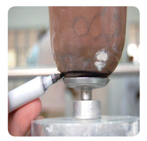
Secure the heavy-duty nut with a self-tapping screw (4 mm x 30 mm)
